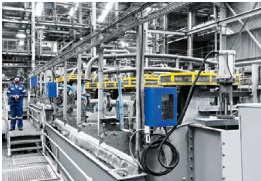
Picture: Flotation cells in a mineral processing facility
